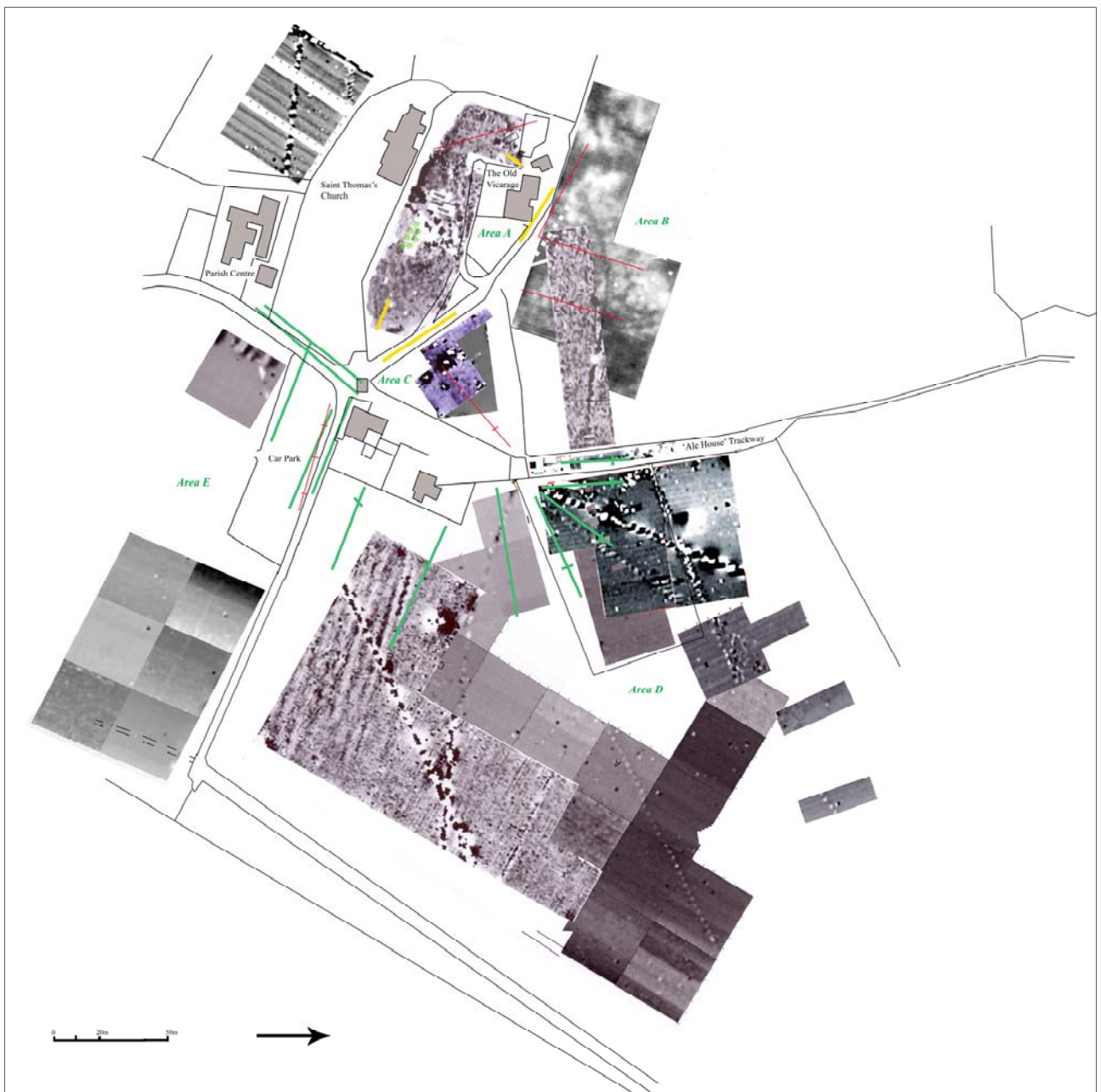
Fig 2.3: A plan showing the current extent of the geophysical survey. The coloured lines represent coverage by Ground Penetrating Radar (GPR).
